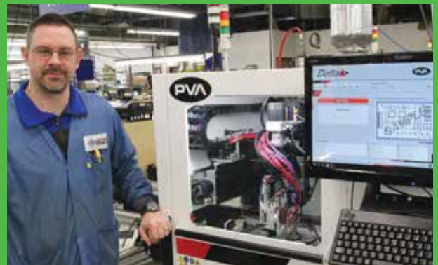
Manufacturing Engineer Hans Haase with the new PVA Delta 6 conformal coating machine.
