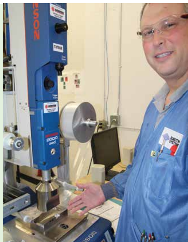
At right, Senior Technical Support Engineer James Pickering shows off Electronic Systems' new ultrasonic welder.
