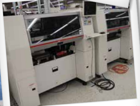
Newly purchased Samsung SM481 and 482 expand surface mount capabilities on the main production floor.
