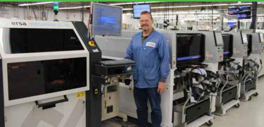
With the recent investment in three new Fuji AIMEX III surface mount placement machines and an ERSA Versa Print SI-3D screen printer, Electronic Systems has added capacity and boosted its commitment to quality.
