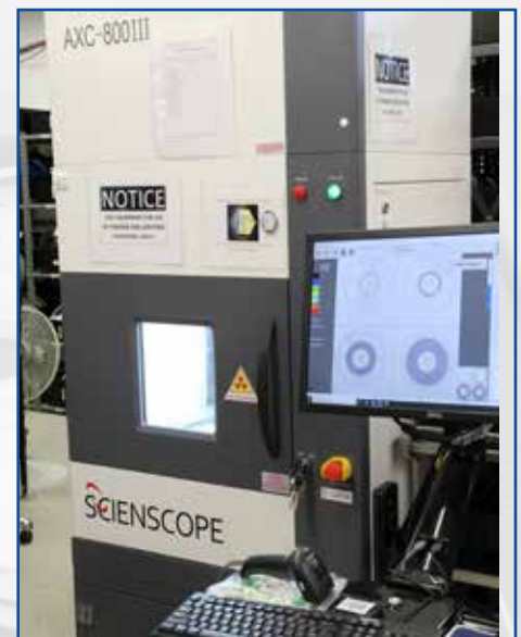
ESI's new Scienscope X-ray Component Counter can accurately count tens of thousands of components in seconds.
